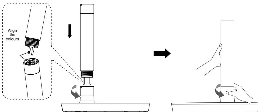
To attach the column/s and air circulator head align the gold metal guide pin with the gold hole and insert to bring the poles together. Turn the security collar counter clockwise until it is securely tightened.
