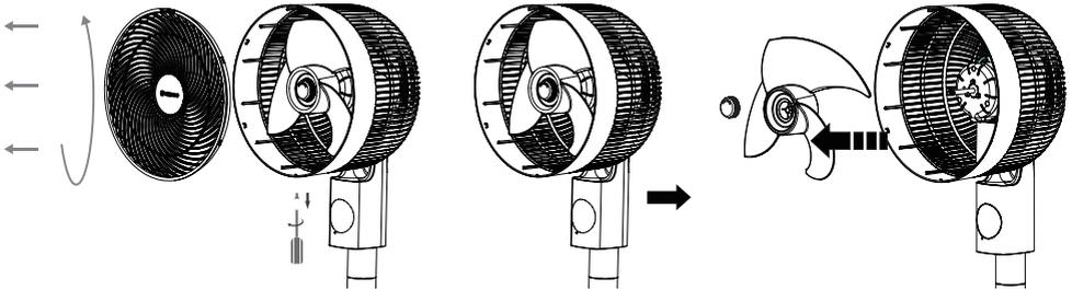
1. Using a screwdriver, unscrew the screw at the bottom of the air circulator head.
