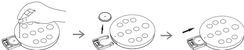
If the remote control fails to work within 4 metres of the air circulator, replace the battery. Battery type: CR2025 or CR2032. To replace the battery follow the steps below:
