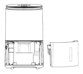
Step 1: Remove the water tank.
